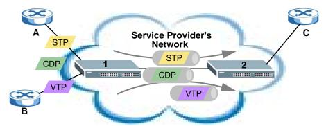
In the following example, if you enable L2PT for STP, you can have switches **A**, **B**, **C** and **D** in the same spanning tree, even though switch **A** is not directly connected to switches **B**, **C** and **D**. Topology change information can be propagated throughout the service provider's network.
