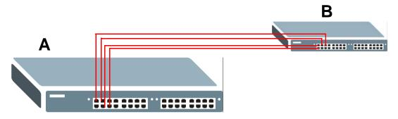
2 Configure static trunking - Click Advanced Application > Link Aggregation > Link Aggregation Setting. In this screen activate trunk group T1, select the traffic distribution algorithm used by this group and select the ports that should belong to this group as shown in the figure below. Click Apply when you are done.
