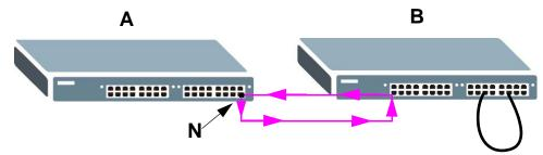
The loop guard feature checks to see if a loop guard enabled port is connected to a switch in loop state. This is accomplished by periodically sending a probe packet and seeing if the packet returns on the same port. If this is the case, the Switch will shut down the port connected to the switch in loop state.
