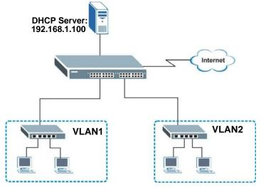
Configure the **DHCP Relay** screen as shown. Make sure you select a DHCP option 82 profile (**default1** in this example) to set the Switch to send additional information (such as the VLAN ID) together with the DHCP requests to the DHCP server. This allows the DHCP server to assign the appropriate IP address according to the VLAN ID.
