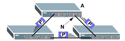
Note: After resolving the loop problem on your network you can re-activate the disabled port via the web configurator (see Section 8.7 on page 72) or via commands (See the CLI Reference Guide).
