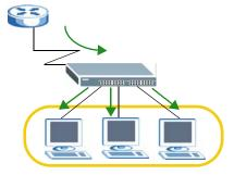
Figure 88 Static Multicast Forwarding to A Single Port
