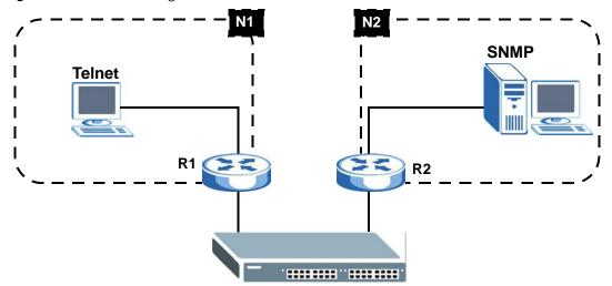
Figure 227 Static Routing Overview
