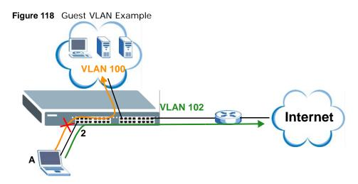
Use this screen to enable and assign a guest VLAN to a port. In the **Port Authentication >** 802.1x screen click **Guest VIan** to display the configuration screen as shown.
