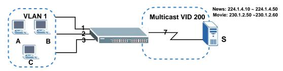
To configure the MVR settings on the Switch, create a multicast VLAN in the **MVR** screen and set the receiver and source ports.
