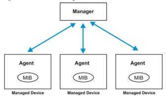
An SNMP managed network consists of two main components: agents and a manager.
