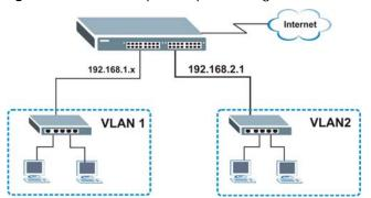
Figure 30 Initial Setup Example: Management IP Address
