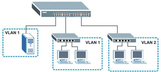
Figure 4 Shared Server Using VLAN Example
