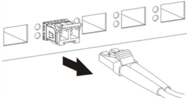
**Figure 16** Opening the Transceiver's Latch Example
