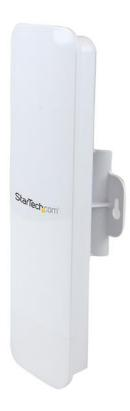
The R300WN22OP5E Outdoor Wireless Access Point lets you create or extend the range of a 5GHz Wireless-N (300Mbps) network to an outdoor location, letting your wireless devices connect to your network with enhanced reliability and speed, with less network congestion.
