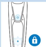
*Note:* You can also deactivate the travel lock by connecting the appliance to the mains.
