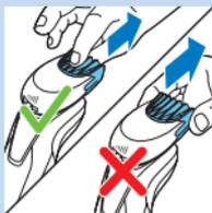
*Note: Grab the comb in the centre to pull it off the beard styler attachment. Do not pull at the sides of the comb.*
