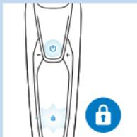
While you activate the travel lock, the travel lock symbol lights up white continuously. When the travel lock is activated, the shaver produces a sound and the travel lock symbol flashes.
