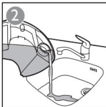
**EN** Clean the appliance and wipe any deposits off the steamer head with a damp cloth and a non-abrasive liquid cleaning agent.
