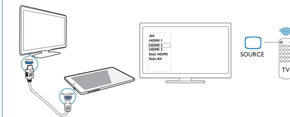
EN Use an HDMI cable to connect PI3910 with an HDTV. On the remote control of the TV, use the source button to select the HDMI input connector that connects PI3910.
