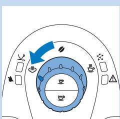
If you want to froth milk after switching on the machine or after brewing a cup of coffee, there may still be some water in the internal circuit. You need to let this water flow out of the machine first.
