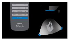
An advanced spatial calibration function developed by our unique innovation lab ensures the best possible balance of sound, regardless of where in a room rear speakers have been placed. When triggered, this function uses a specially designed tonal signal to locate each of the rear speakers. It then uses this information to identify the best sound balance for this speaker placement and adjusts the sound of each speaker to match. This allows the listener to enjoy properly balanced
