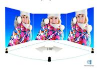
IPS-AHVA displays use an advanced technology which gives you extra wide viewing angles of 178/178 degree, making it possible to view the display from almost any angle. Unlike standard TN panels, IPS-AHVA displays give you remarkably crisp images with vivid colors, making it ideal not only for Photos, movies and web browsing, but also for professional applications which demand color accuracy and consistent brightness at all times.
