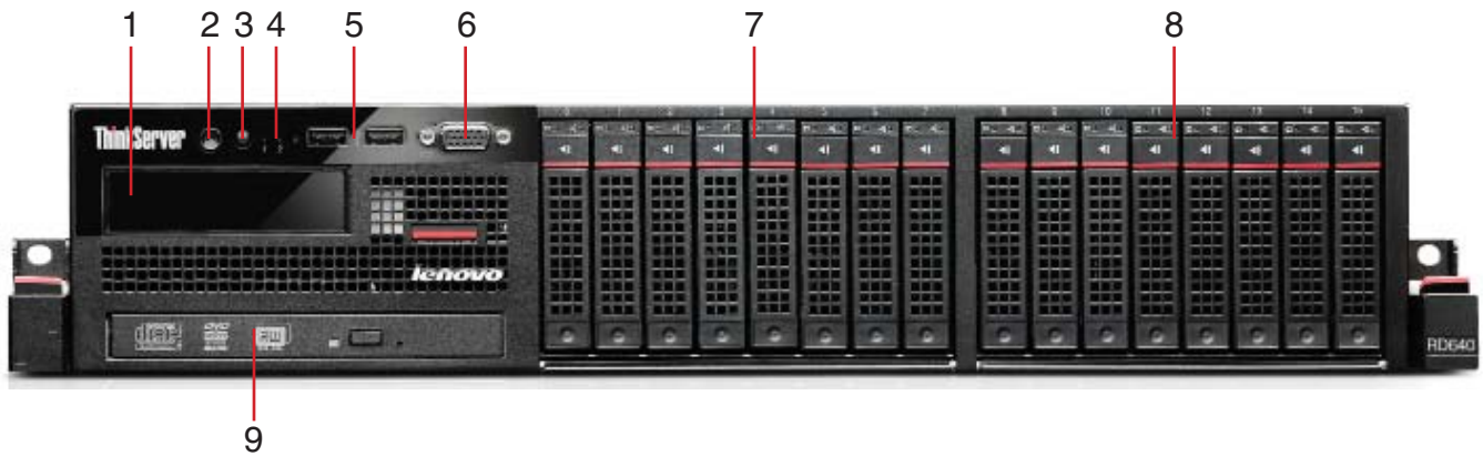
ThinkServer RD640 with 8x2.5"/16x2.5" Disk Drive Bays
