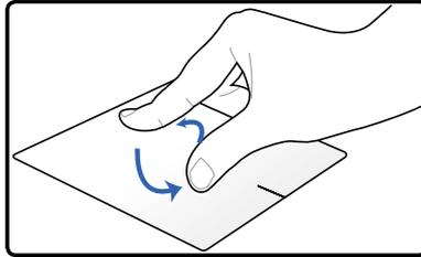
Put two fingers on the touchpad then turn in a circular motion, either clockwise or counterclockwise, to rotate an image.
