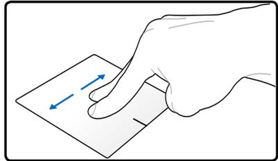
To enable continuous scrolling, hold your fingers on the edge of the touchpad when moving from up to down/left to right and vice versa. The mouse pointer changes to a double-headed arrow pointer
