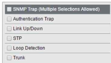
The image shows a configuration form titled "SNMP Trap (Multiple Selections Allowed)". It contains five rows, each with a checkbox and a label: "Authentication Trap", "Link Up/Down", "STP", "Loop Detection", and "Trunk". All checkboxes are currently unchecked.
