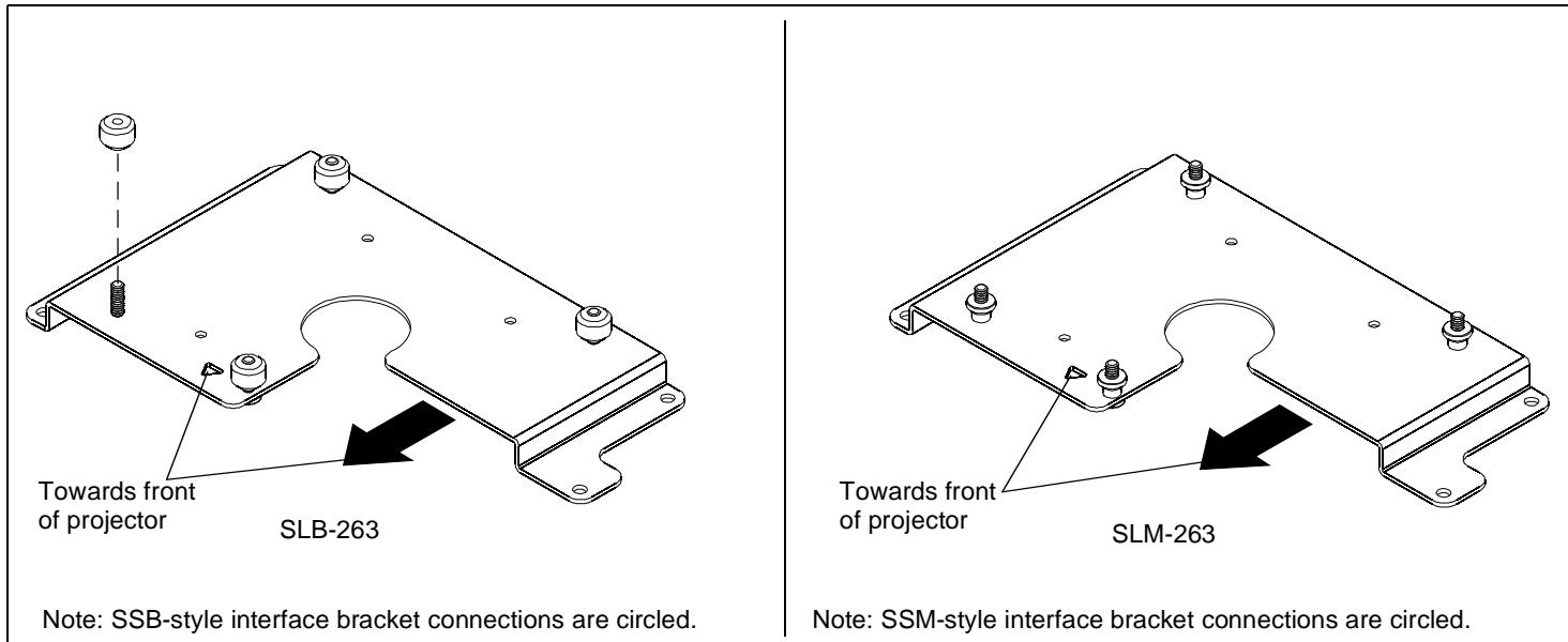
Note: SSB-style interface bracket connections are circled.
