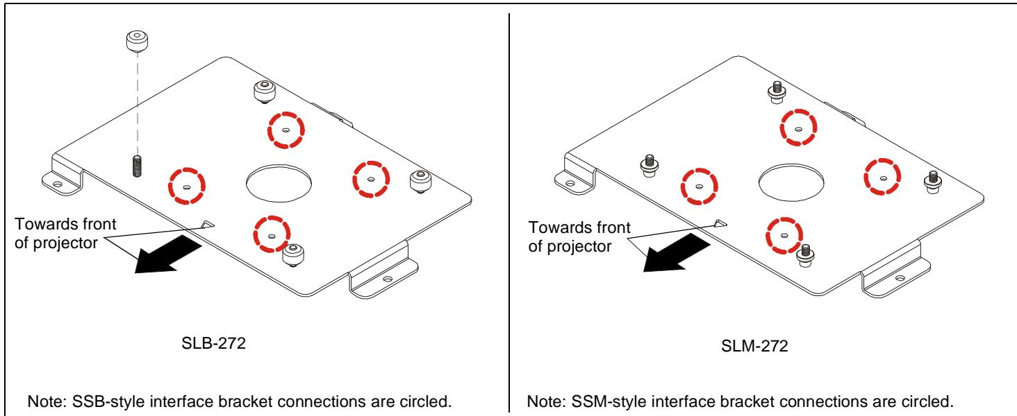
Note: SSB-style interface bracket connections are circled.
