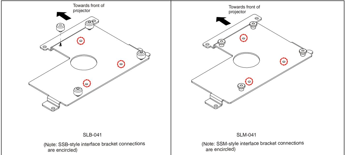
\*\*Only used when installing SLB/SSB interface brackets.
