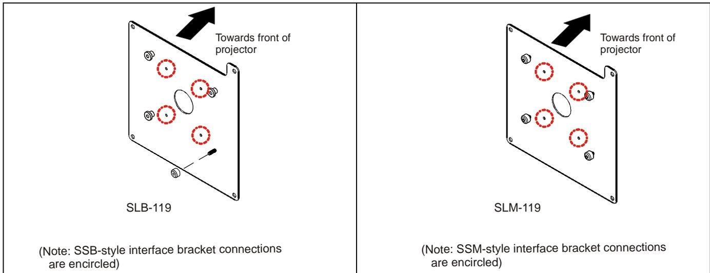
\*\*Only used when installing SLB/SSB interface brackets.
