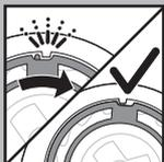
NOTE: Each retaining ring has two recesses that fit exactly into the projections of the shaving head holder. Turn the ring clockwise until you hear a click to indicate the ring is fixed into place.
