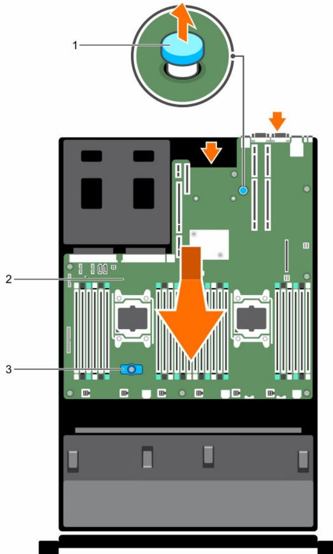
**Figure 46. Removing and installing the system board**
