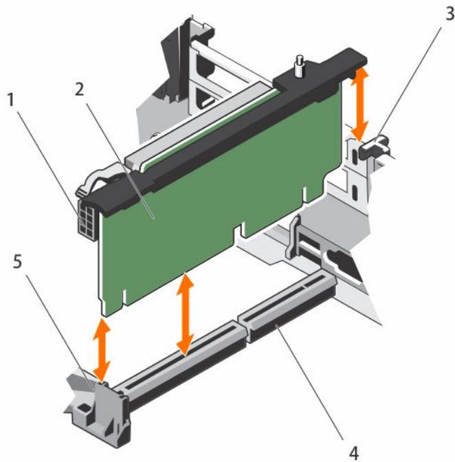
**Figure 25. Removing and installing the expansion card riser 2**
