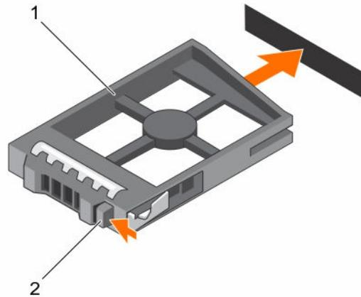
**Figure 10. Removing and installing a 2.5 inch hard-drive blank**
