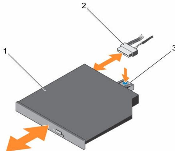
**Figure 13. Removing and installing the optical drive**
