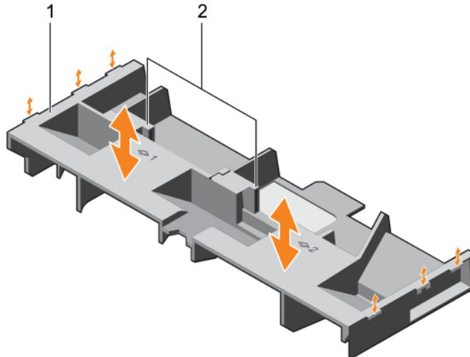
Figure 7. Removing and installing the cooling shroud
