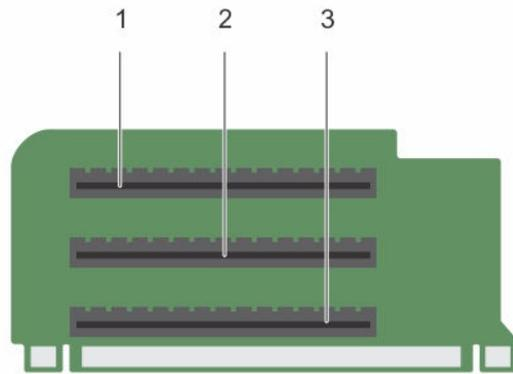
**Figure 24. Identifying connectors on the expansion card riser 1**
