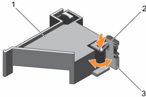
**Figure 18. Opening and closing the PCIe card holder latch**
