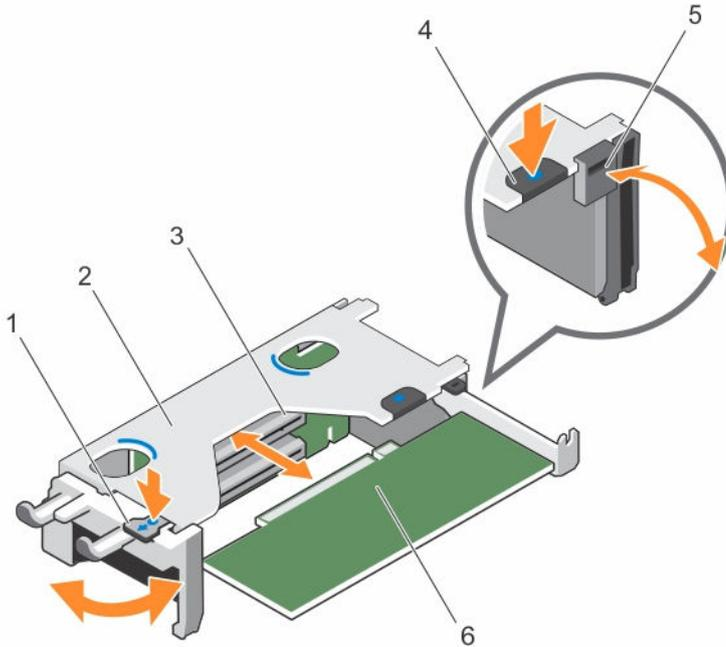
**Figure 21. Removing and installing an expansion-card from expansion-card riser 1**
