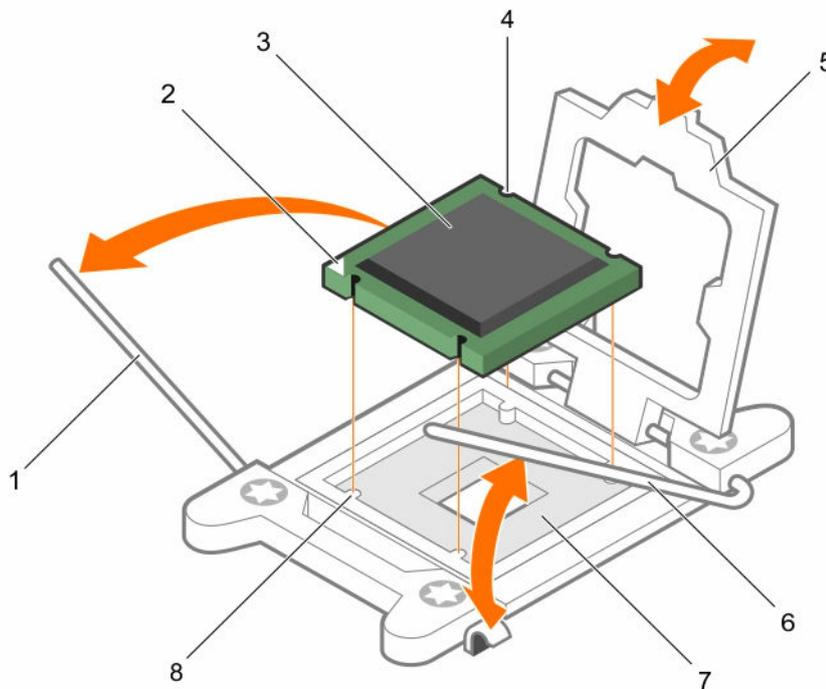
**Figure 37. Removing and installing a processor**
