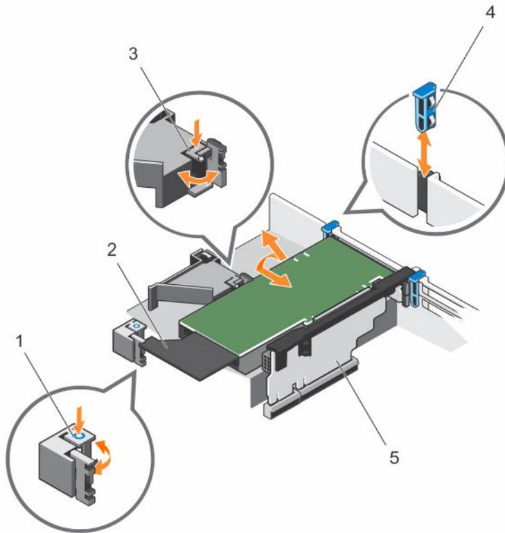
**Figure 30. Removing and installing the GPU card**
