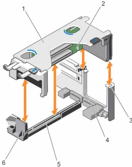
**Figure 23. Removing and installing the expansion card riser 1**
