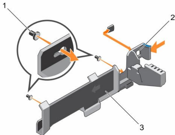
**Figure 19. Removing and installing the cable retention bracket**
