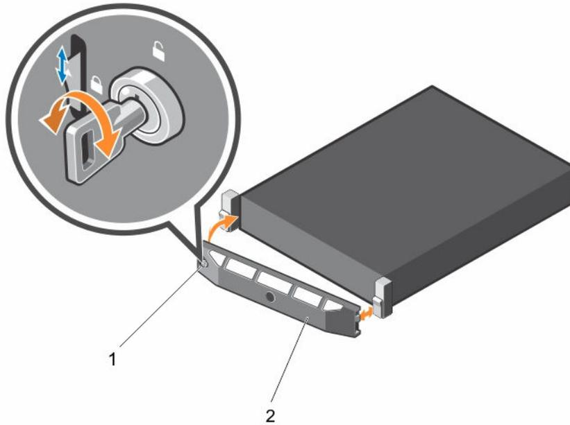
**Figure 5. Removing and installing the front bezel**
