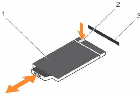
**Figure 45. Removing and installing the information tag**
