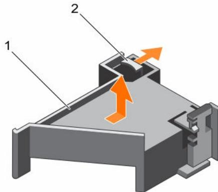
**Figure 17. Removing and installing the PCIe card holder**
