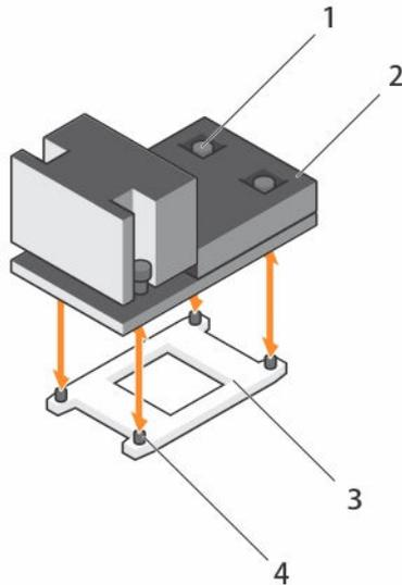
**Figure 35. Removing and installing a processor heat sink**
