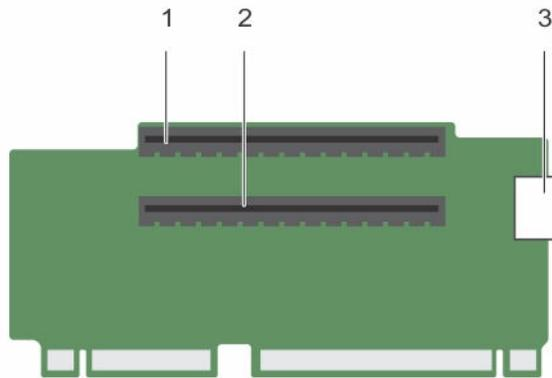
**Figure 26. Identifying connectors on the expansion card riser 2**
