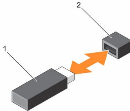
**Figure 16. Replacing the internal USB key**
