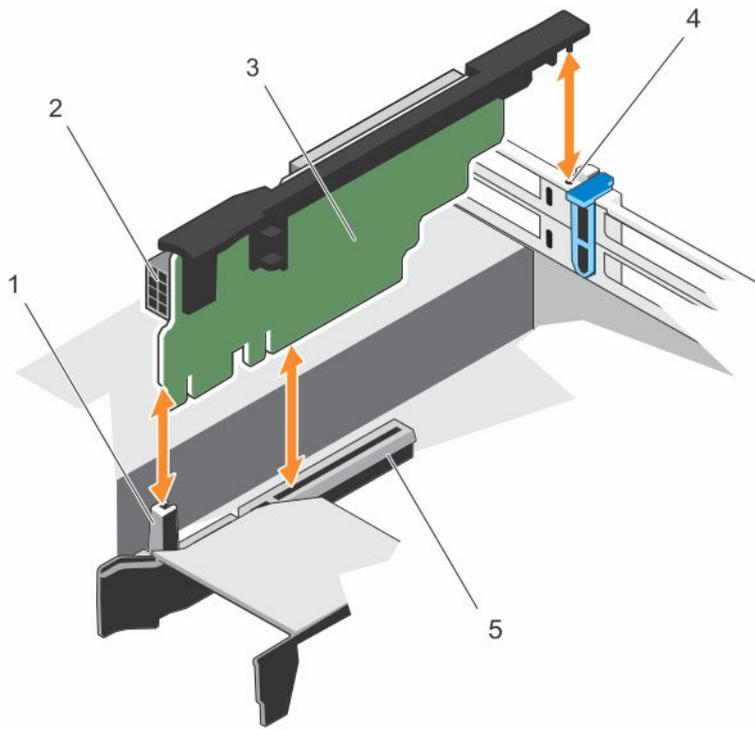
**Figure 27. Removing and installing the expansion card riser 3**
