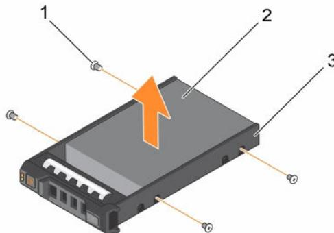
Figure 12. Removing and installing a hard drive into a hard-drive carrier
