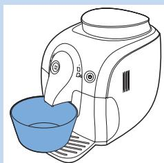
When the machine has heated up, it performs an automatic rinsing cycle to clean the internal circuit with fresh water. This takes approximately one minute.
