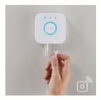
Connect your Philips Hue lights with the bridge to control your lights from your smartphone or tablet via the Philips Hue app. Or control your Philips Hue lights with the Philips Hue dimmer switch for on/off and dimming functionalities or to cycle through the light recipes.
