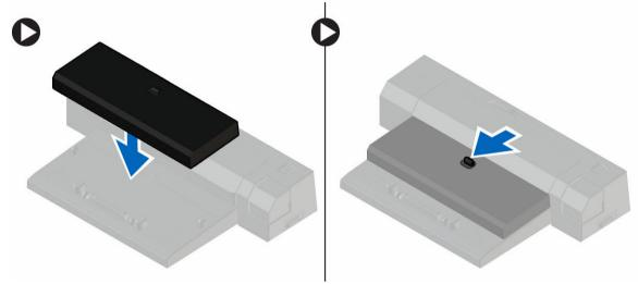
**NOTE:** This docking spacer can be used to dock only the Latitude E7250 / Latitude E7450 computers. You cannot dock any other Dell computers using this docking station.
