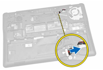
**4.** Disconnect the speaker cable [1] and SIM board cable [2] [3] from their connectors on the system board.
