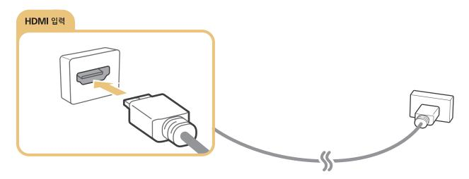
Set Edit Device Type to DVI PC for a computer connected with a HDMI-to-DVI cable, and PC for a computer connected with HDMI cable. Also, set Edit Device Type to DVI Device for an A/V device with a HDMI-to-DVI cable.
