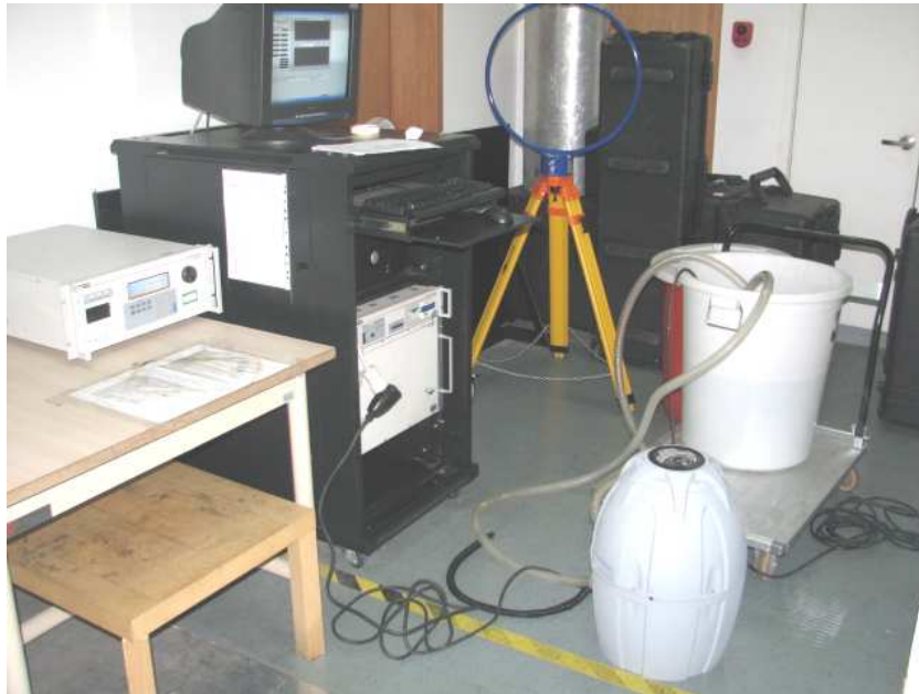
Photograph 2: Set-up for disturbance voltage
