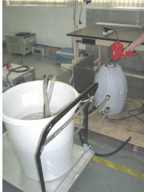
Photograph 6: Set-up for immunity test of surge on AC power line
