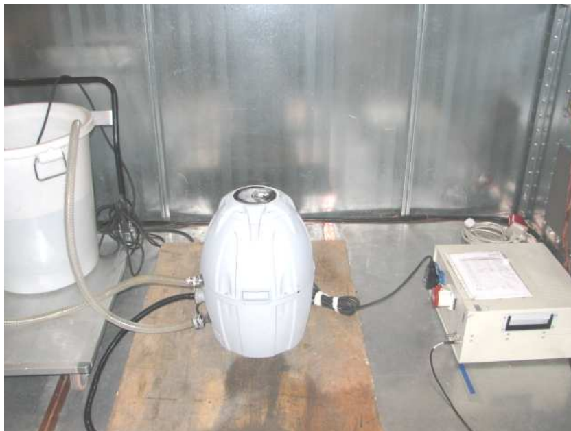
Photograph 2: Set-up for disturbance voltage
