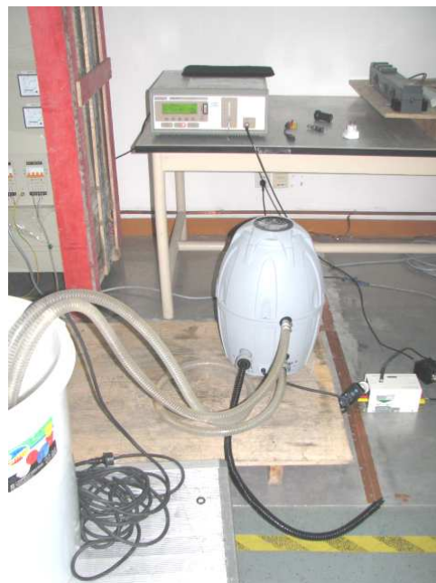
Photograph 8: Set-up for immunity test of injected current on AC power line
