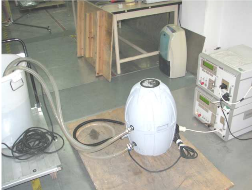
Photograph 8: Set-up for immunity test of injected current on AC power line
