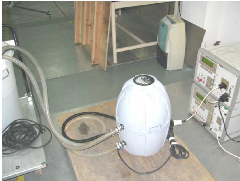
Photograph 6: Set-up for immunity test of surge on AC power line
