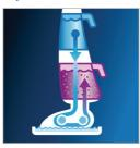
Separate clean and dirty water tanks ensure that you always mop with clean water, all dirt and allergens are contained in the dirty water tank.
