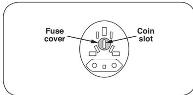
The International Travel Plug Adapter comes with a fuse installed and an extra fuse located in the adapter cap. Use only T2.5A fuses with the International Travel Plug Adapter.
