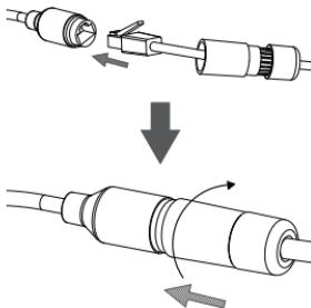
Turn the back part of the waterproof connector clockwise until there is a tight seal around the Ethernet cable.
