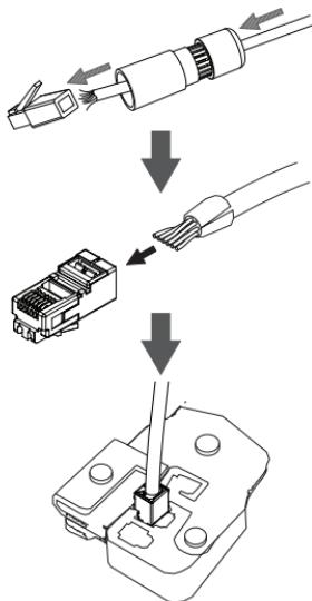
Connect the RJ-45 plug into the Ethernet connector, then screw the waterproof connector to the Ethernet connector by turning it about a half-turn clockwise.
