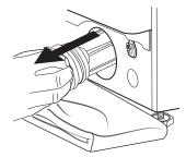
**5.** Clean the water filter: remove residues in the filter and clean it under running water.
