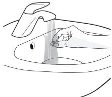
4. Insert the mesh filter again. Connect the inlet hose to water tap and washing machine again. Do not use a tool to connect the inlet hose. Open the water tap and check that all connections are tight.
