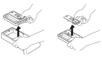
**3.** Clean all parts under running water, removing all detergent or softener residues.
