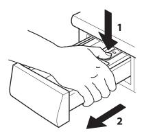
**2.** Remove the insert from the detergent dispenser, as well as the insert of the softener compartment.
