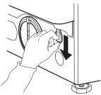
**4.** Afterwards fix the strap again by firmly turning in the screw with the screwdriver.
