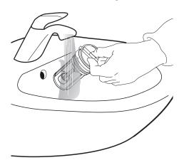
**6.** Insert the water filter and reinstall the plinth: Reinsert the water filter again by turning it in clockwise direction. Make sure to turn it in as far as it goes; the filter handle must be in vertical position. To test water tightness of the water filter, you can pour about 1 liter of water into the detergent dispenser.
