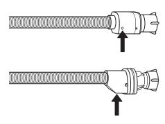
For water stop hoses: check the small safety valve inspection window (see arrow). If it is red, the water stop function was triggered, and the hose must be replaced by a new one.
