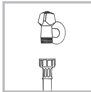
1. Connect the inlet hose by screwing it to a cold water tap using a 3/4 gas threaded connection (see figure).
