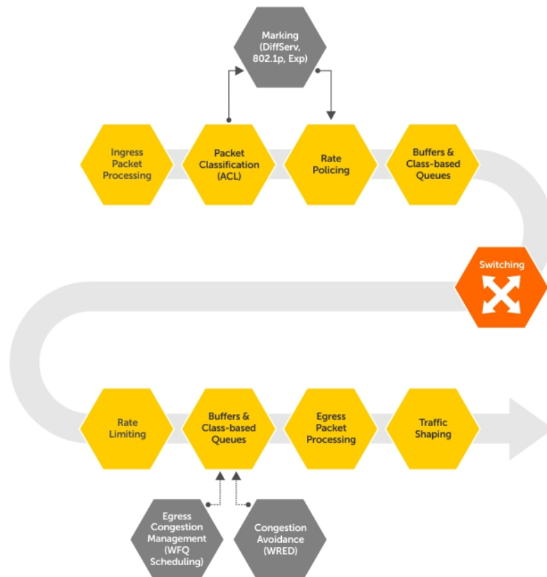
Figure 114. Dell EMC Networking QoS Architecture
