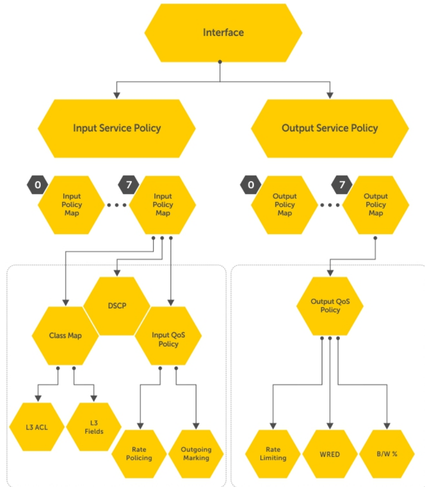
Figure 115. Constructing Policy-Based QoS Configurations
