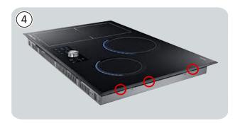
Disassembly of the Assy Control Panel.
