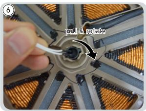
Disassembly of the the PBA.
