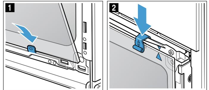
3. Insert the front panel downwards into the retainers (fig. 3).
