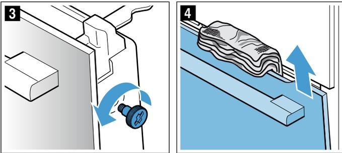
6. Push both retainers at the top of the intermediate panel upwards, but do not remove them (fig. 5). Hold the panel with one hand. Take out the panel.
