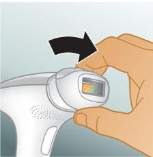
To remove the attachment, pull it off the light exit window.
