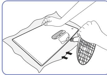
Hold the main body of the product with your hand as shown by the figure. Push the assembled stand into the main body in the direction of the arrow as shown in the figure.
