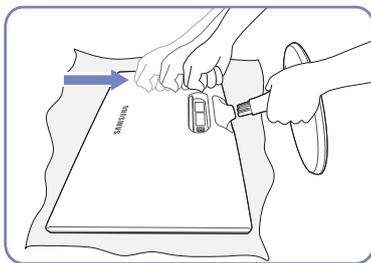
While holding the stand neck with one hand, pound the other fist down onto the top of the stand base in the direction of the arrow to detach the stand base.
