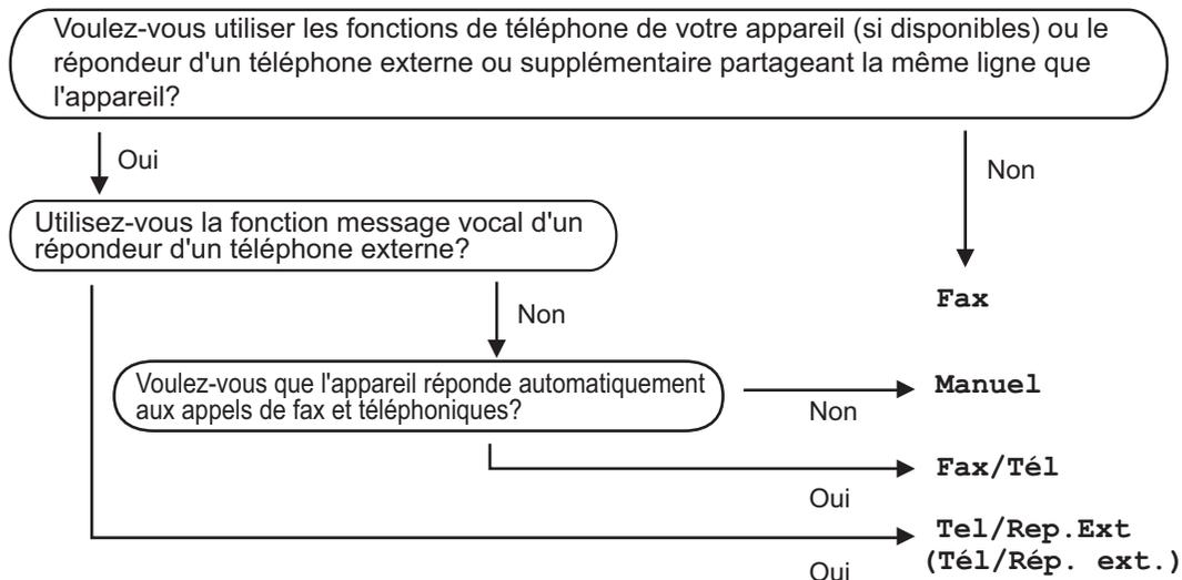
**1** Appuyez sur
