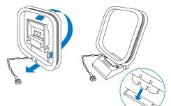
2 Connect the AM loop antenna to the AM jack on the back of the main unit.
