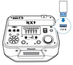
Insert the USB plug of the device into the **USB B** socket.
