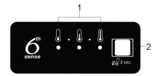
1. Indicator Leds (to display the current temperature setpoint or the Fast Cooling function) 2. Fast Cooling Button / Temperature Button
