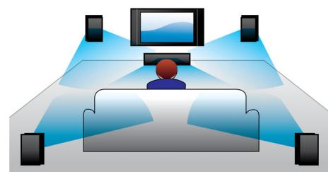
A built-in Dolby Digital decoder eliminates the need for an external decoder by processing all six channels of audio information to provide a surround sound experience and an astoundingly natural sense of ambience and dynamic realism. Dolby Pro Logic II provides five channels of surround processing from any stereo source.
