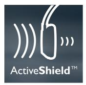
ActiveShield<sup>™</sup> active noise canceling techonolgy features two feed-backward microphones used for canceling low frequencies. It detects ambient noise and inverting the sound wave, effectively cancelling it out and converting background noise to silence.
