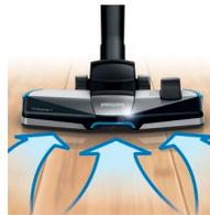
The TriActive+ nozzle applies 3 cleaning actions in one go: 1) It gently opens the carpet with its specially designed soleplate to remove the dust deep down. 2) It sucks up big bits with its larger opening at the front. 3) It sweeps up the dust and dirt alongside furniture and walls with its two side brushes.
