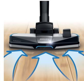
The TriActive+ nozzle applies 3 cleaning actions in one go: 1) It gently opens the carpet with its specially designed soleplate to remove the dust deep down. 2) It sucks up big bits with its larger opening at the front. 3) It sweeps up the dust and dirt alongside furniture and walls with its two side brushes.
