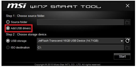
Plug in the bootable Win 7 USB pen drive, click to locate the device.
