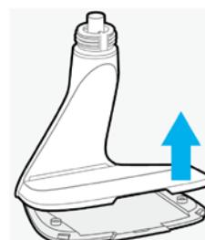
3. Drill two mounting holes and fix the mounting base.
