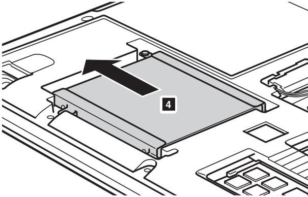
⑦ Take out the hard disk drive secured in a metal frame **5**.
