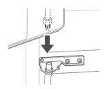
2 Fit the hinge over the hinge lever latch and slot it into place. Rotate the lever clockwise 2 and fasten the hinge.
