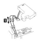
3 Rotate the hinge lever 1 clockwise. Lift the top hinge 2 free of the hinge lever latch.
