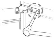
Twist the hinge to raise the pivoting end so that the door can be lifted off.
