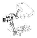
4 Make sure that the door-switch located inside the cover is tightly connected. Position the cover in its place. Insert and tighten the cover screw 2.
