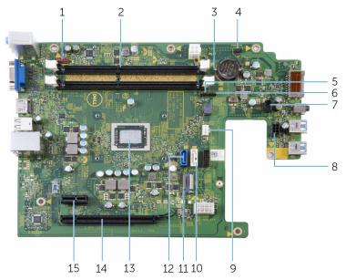
chassis-fan cable connector 1 2 memory-module slots (2) 3 4 coin-cell battery power-button cable connector 5 CMOS jumper 6 password jumper 7 lighting-cable connector 8 drive power-cable connector 9 processor-fan cable connector 10 optical-drive/hard-drive 2 data
