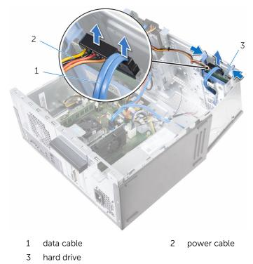
4 Spread apart the hard-drive bracket from one edge and lift the hard drive up.
