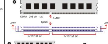
3. Check that the latches are closed, and the memory module is firmly installed.
