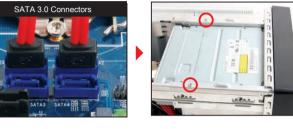
5. Connect the Serial ATA and power cables to the HDD.
