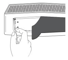
In case that the unit freezes due to malfunction, remove the rubber sleeve and press the reset hole using an object like a thin pin. Then the unit is turned off completely.
