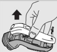
Do not connect the shaver to the mains again after the battery has been removed.
