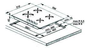
NOTE: if the distance "A" between the wall cabinets is between 600 mm and 730 mm, the height "B" must be a minimum of 530 mm. If the distance "A" between the wall cabinets is greater than the width of the cooktop, the height "B" must be a minimum of 400 mm. In case of installation of a hood above the cooktop, please refer to the hood instructions for the correct distance.
