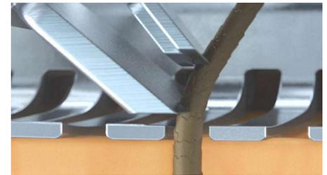
Shave closer with the dual-blade Super Lift & Cut Action. The first blade raises each hair while the second blade comfortably cuts below skin level, for exceptionally smooth results.
